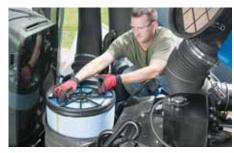
The large and extra-large frame tractors feature a new engine air intake system. The engine air filter has been relocated under the hood for a more efficient air flow and filter life.
